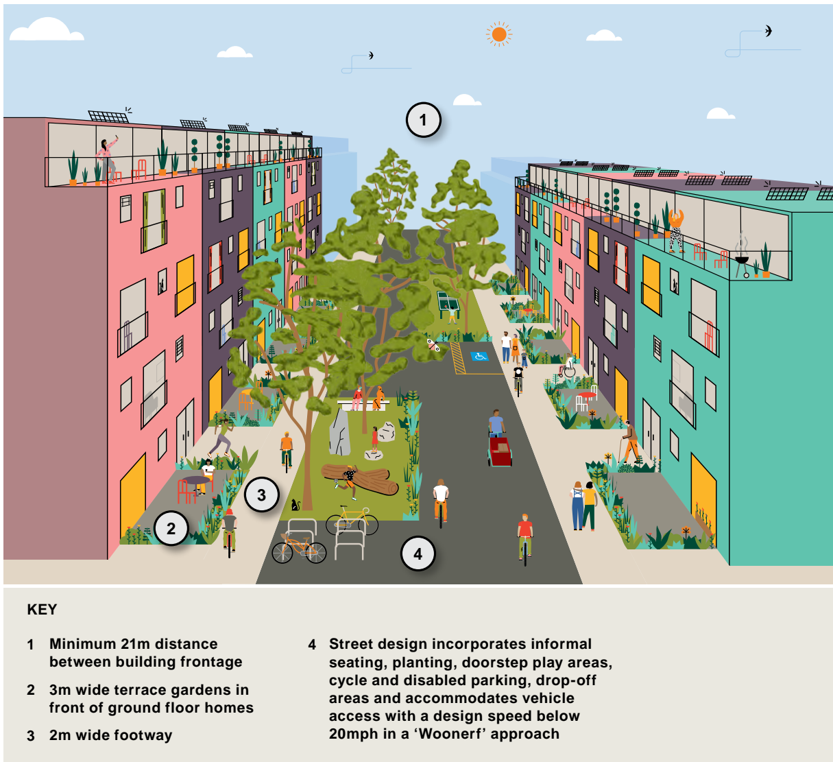
Figure 18: Illustration of proposed design features for secondary streets in medium density areas
